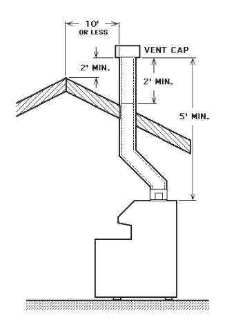
Fig. 5: Minimum Venting Measurements
